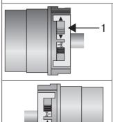
Switch the direction switch (1) to the opposite position.
